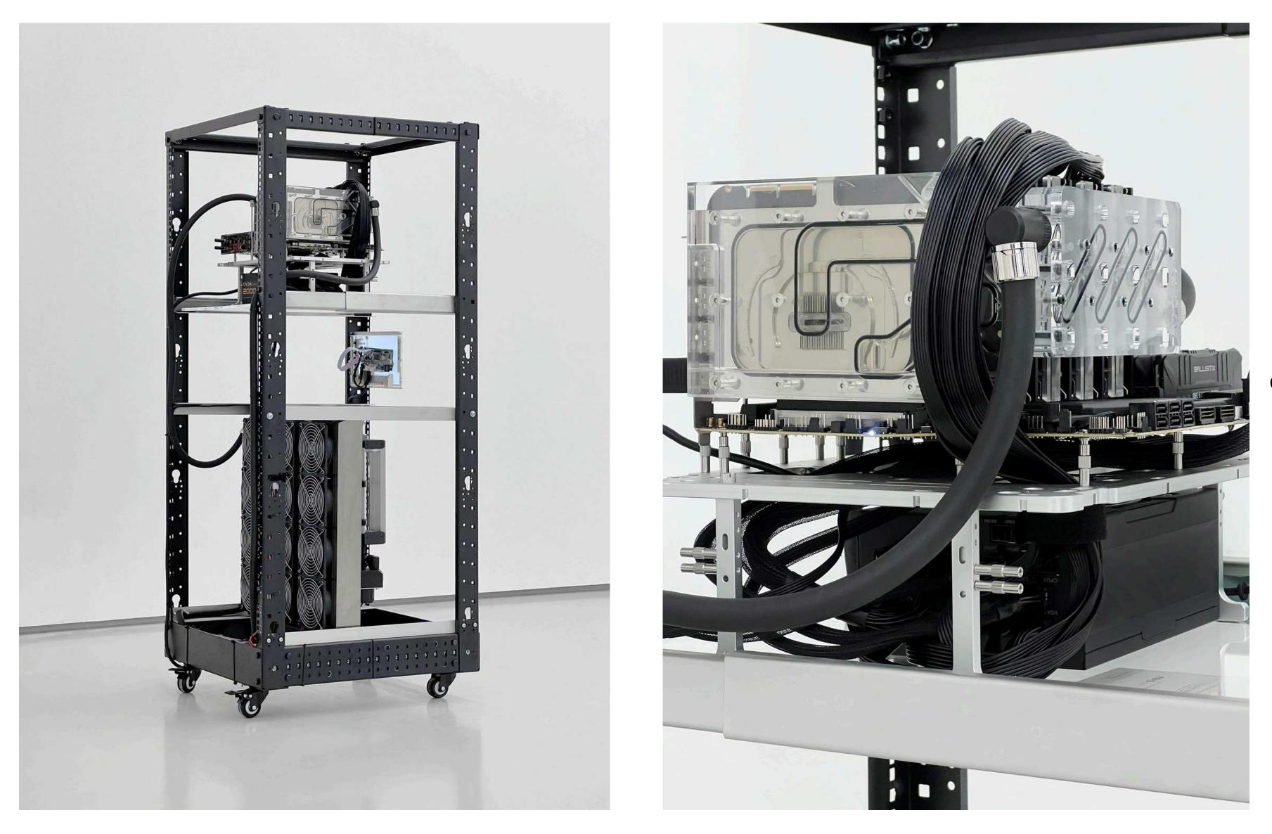
EnBW (client of Gazprom Germania) electricity contract, rack case, open frame server including four Nvidia 3090 GPUs, custom water loop, Ethereum Blockchain
